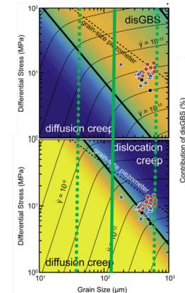
Figure 7<sup>[3]</sup>: (Top) Wet and (Bottom) Dry Mechanics of Deformation from Nevitt et al. 2019<sup>[3]</sup>. Plotted with grain size (um) and Differential Stress (Mpa) Green lines are range and mean of mylonite zone.
